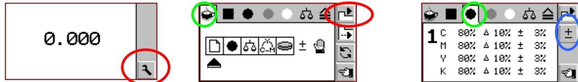
Select the icons marked in red with the UP and DOWN buttons, click ENTER activate them. Use the TAB SHEET SELECT tool to move from the AUTO tab to the DOT GAIN tab marked in green. Select the EDIT icon marked in blue with the UP and DOWN buttons, click ENTER to activate it.
