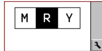
**EFFICIENCY** is a measure of how well the second ink is trapped to the first in relation to how well that ink transfers to dry paper. Low Trapping Efficiency causes red, green, or blue overprint colors to reproduce poorly. Place the aperture on a Trap target. Press the head down and watch the display. The HISTORY STACK is replaced by a group of three large color icons.
